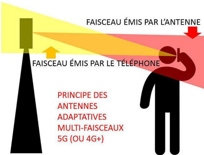
**USAGE D'ANTENNES ADAPTATIVES MULTI-FAISCEAUX MULTI-CANAUX (MIMO)**
